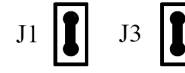
(d) J1, J3 short circuit CW/CCW mode and active at high level (The fixed level)
