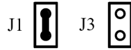
(c) J1 short circuit, J3 open circuit CW/CCW mode and active at low level (The fixed level)
